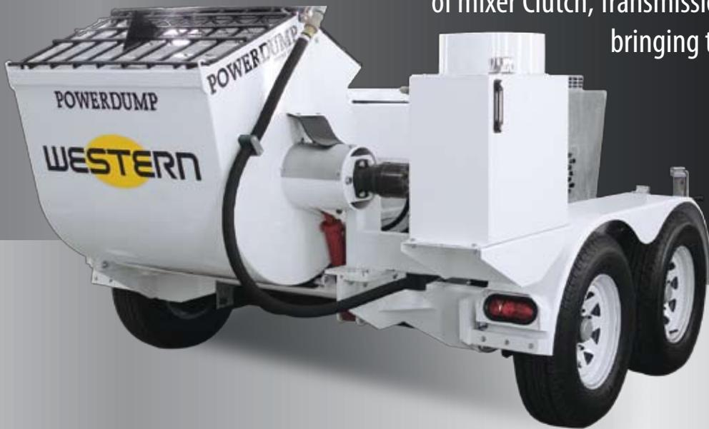
Offset pivot point allows for LOWEST charging height available which combined with the hydraulic POWERDUMP system increases operator and crew's total productivity.
