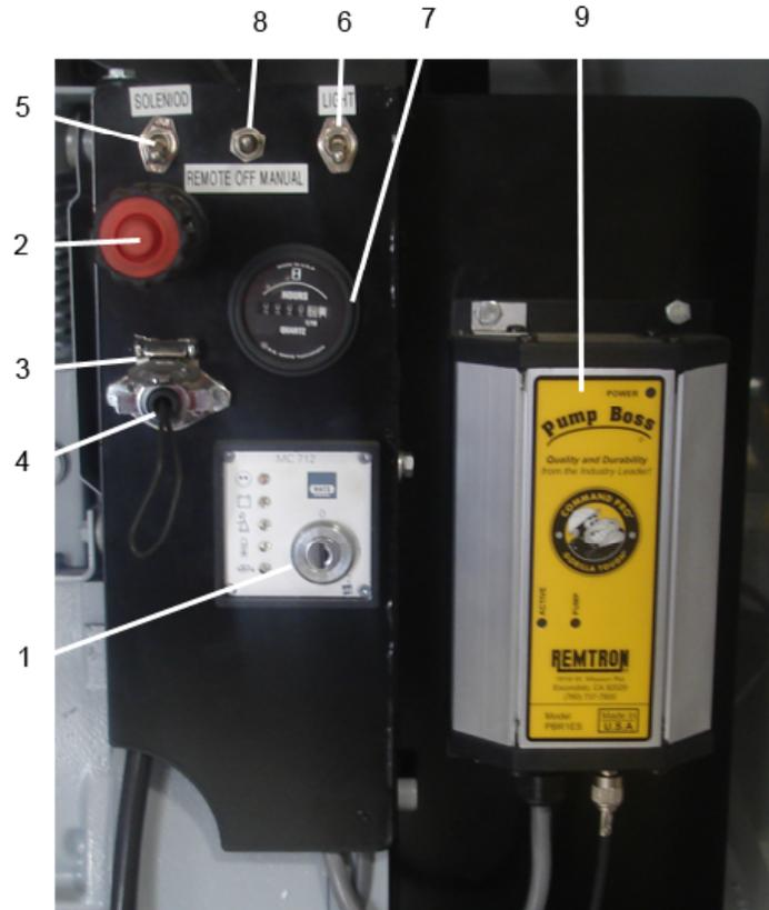
1. **IGNITION BOX** – A 3 position key switch used to start and stop engine. Turning key to the right starts engine, release key for run position and turn to LEFT to stop engine. Box includes light indicators for charging system, oil level, temperature and fan belt. (see engine manual for more details)
